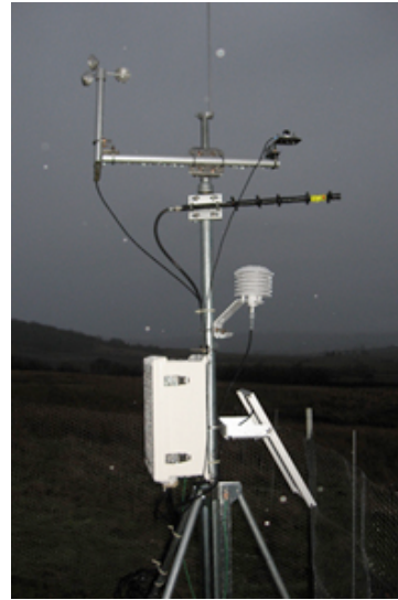
Figure 1. REAP weather station. Pictured from left to right, starting at top: anemometer, lightning rod, quantum point sensor, directional antenna, relative humidity and temperature sensor within gill radiation shield, enclosure and solar panel.
